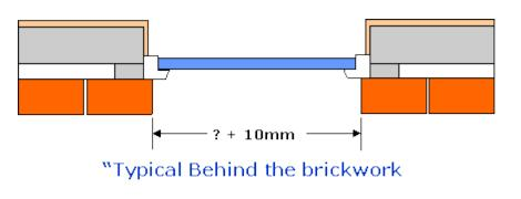
Measuring from the outside, take three different width measurements of the outer brickwork from top middle and bottom of the existing brickwork opening. From the narrowest reading, add 10 mm. If measuring to fit frames in stonework that has irregular shapes, make suitable allowances so that any openers will pass any irregularity of the stonework.
