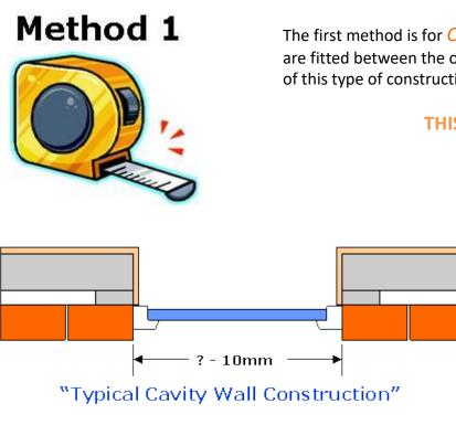
The first method is for *Cavity Wall Construction*, the frames are fitted between the outer skin of brickwork. If your property is of this type of construction then:-
