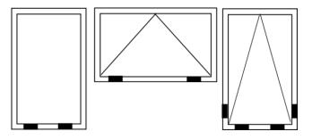
The objective of 'toe & heeling' is to transfer the weight of the glass onto the hinge side of the frame. Correct use of this technique will give trouble free operation once the vents have been set correctly. The vent should be flexed upwards if necessary to allow the insertion of the top packers.
