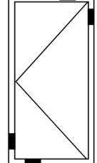
If your door sash is catching at the bottom of the frame you need to LIFT the sash.
